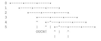
Here we have a collision. Some lines printed in later passes overprint lines printed by earlier passes. We can see why by considering which row number is printed by a given jet number j (numbered from 0) of a given pass, p:
