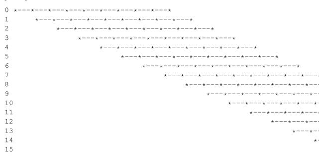
Now we have to determine which line is printed by each jet on each pass. If we number each line generated as we split up a row, we can use these numbers. We'll number the lines in our diagram by replacing the  $\star$ s with integers in the range [0...H-1].
